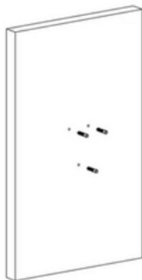
Insert the plastic expansion plugs into the holes
