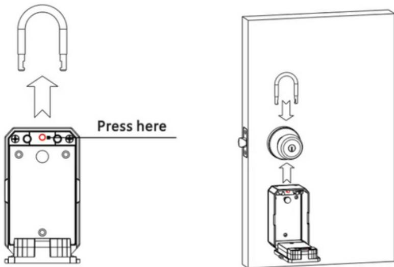
Press the shackle release button inside the device and take off the shackle. Then hang the shackle around the cylindrical lock and clip in the device.
