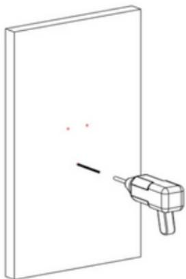
Drill 3 holes into the wall where the screws will line up
