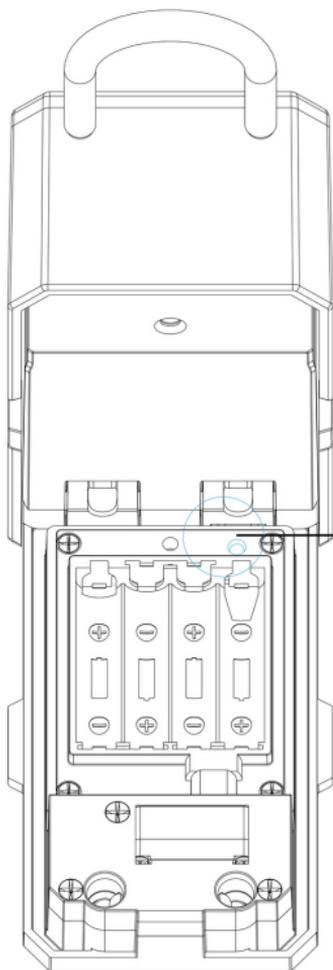
Press and hold the reset button for 2 seconds until you hear "Please enter the initialization password."
